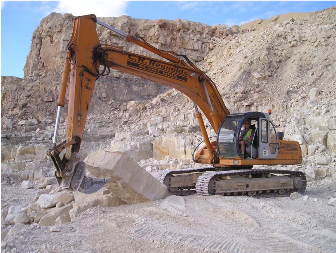
Quarrying limestone for aggregates
